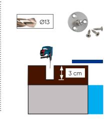
Secure the anchor using the 3 screws supplied.
